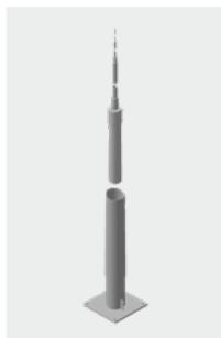
**Telescopic lightning protection mast 13.38 m above ground with screw-in foundation**
