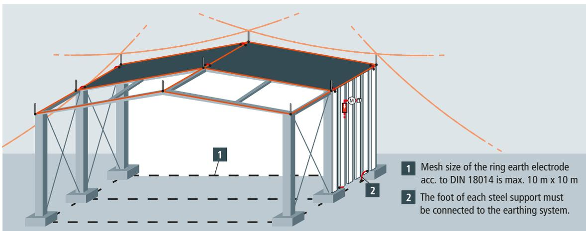
Figure 7 Steel hall with metal cladding and air-termination installed on the foil roof
