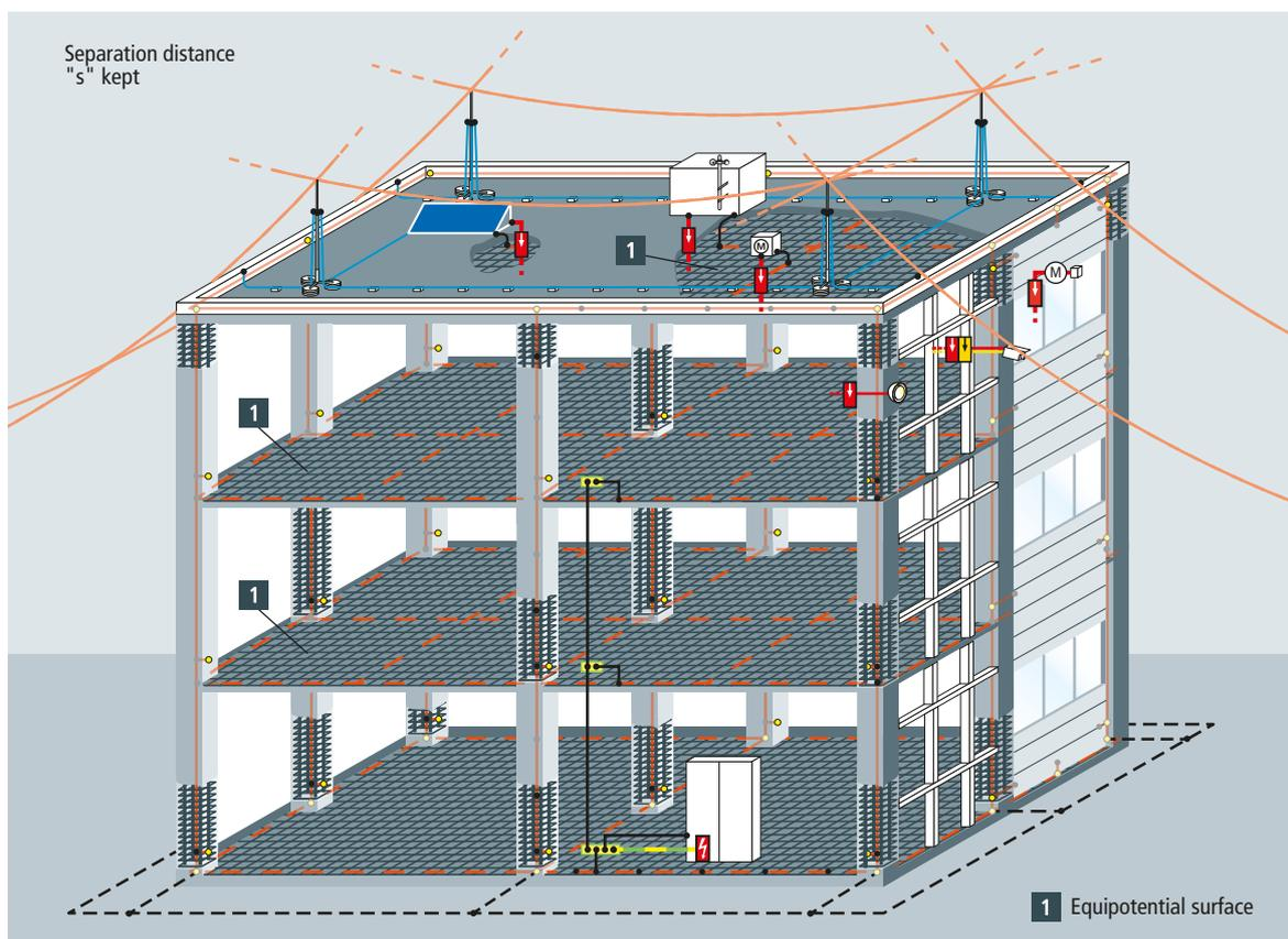
Figure 3 Multi-storey building with equipotential surfaces including air-termination system
