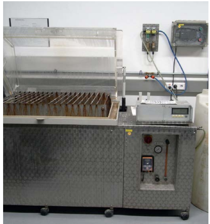
Figure 1: Test in a salt mist chamber.
