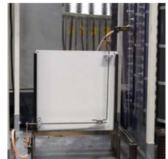
Figure 5: Specimen fixed on insulating plate (MV clamp) for a test in the impulse current laboratory.
