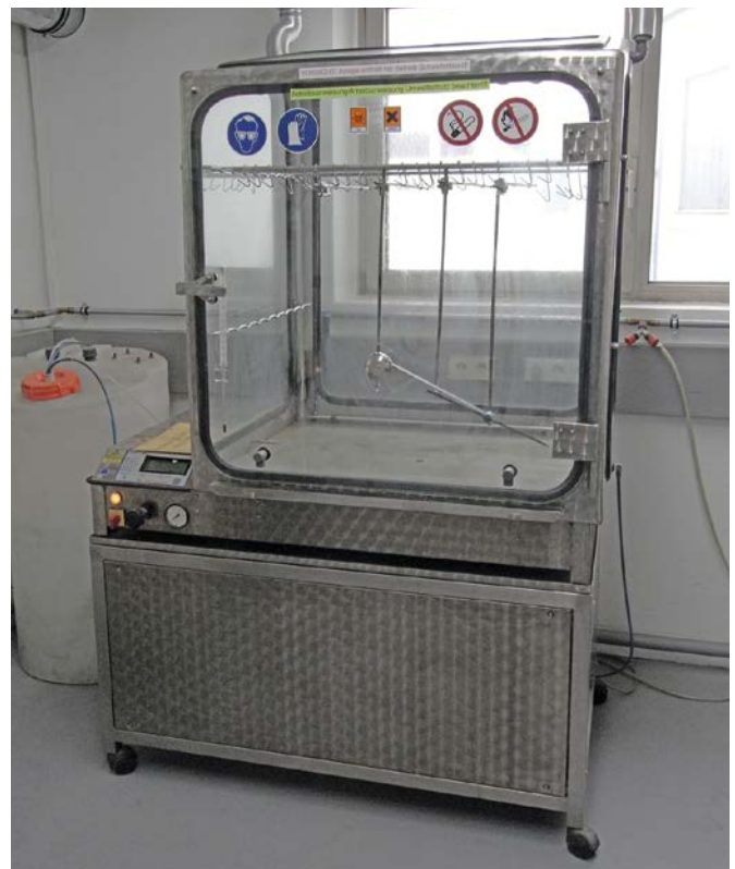
Figure 2: Test in a Kesternich chamber.
